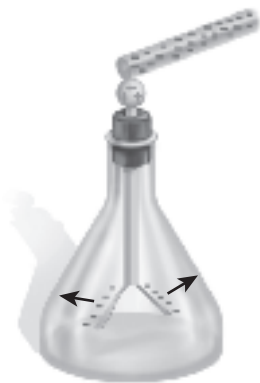
Charging an electroscope by conduction
